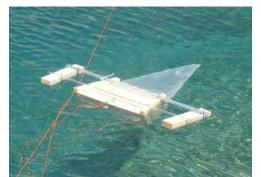
For sampling, a wooden self-constructed LADI-trawl was built. The aim was to have a low-cost, light and easily transportable construction. 60 representative fragments were analysed by means of FT-IR spectroscopy, of which 51 were assigned to 22 different types of plastics. Larger particles, so-called microplastic, were found at 2 locations. Thus, plastic residues were
